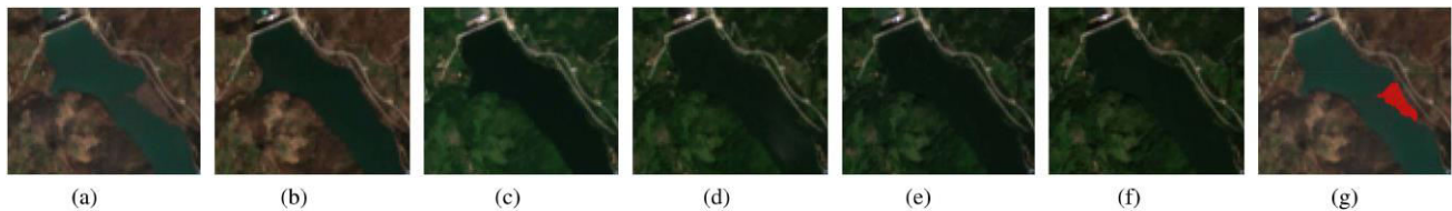
Fig. 3. Plastic candidates identified at dam sites along the Lim river (Serbia). True-color composites of Sentinel-2 subsets from 2020 are shown (refer to Fig. 6 for the full view). Subimages (a)—(f) were captured on the same day as the higher resolution PlanetScope image in the insert of Fig. 6 [(a) 20th March, (b) 9th April, (c) 10th July, (d) 28th July, (e) 22nd August, and (f) 6th September] and the plastic mask derived in (g) aligns with the plastic extent outlined in the PlanetScope image.
